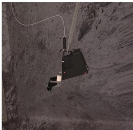
Using the Mounting-hook the trap is lowered down the manhole.
