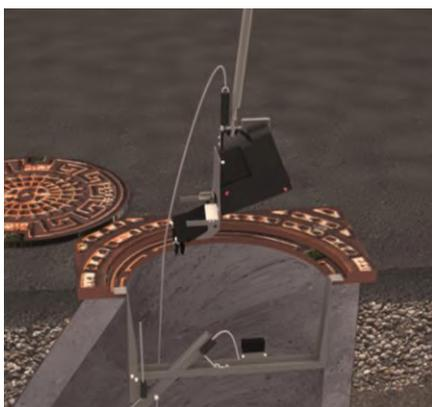
Using the Mounting-hook the trap is lifted up from the manhole
